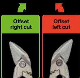
Offset aviation snips allow you to keep your hand on top of the sheet for cuts through the center of the sheet. These tools cut at a sharper angle, distancing your hands from sharp, jagged work surfaces.
